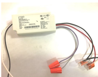
Wiring of One Pendant ESS010W-0500-12
