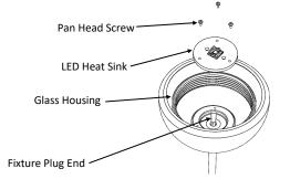
Step 8: If LED has a protective sticker, remove sticker before installing Glass. Screw Glass and Retention assembly fully into Glass Housing.
