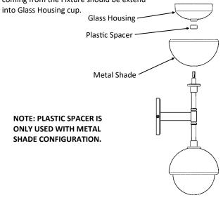
Step 7: Make connection between Plug end connected to LED and Plug end coming from fixture. Attach LED heat sink to Glass Housing with 3X Pan Head screws.
