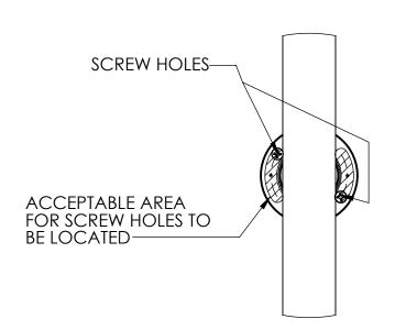
3. CLOCK SCREW HOLES SO THEY ARE NOT COVER BY THE LIGHT BODY. SLIGHTLY LOOSE IS ACCEPTABLE IF THERE IS NO ORIENTATION THAT DOES NOT BLOCK THE SCREW HOLES.
