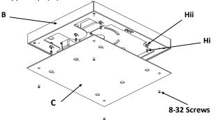
**Step 2:** Mount Canopy (B) to ceiling using the appropriate Hardware Packet (A) and included instructions. Leave Cover Plate (C) hanging.
