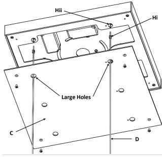
Step 4: Next, pass the Power Cable (E) through the small hole in the Cover Plate (C) and the small hole in the Canopy (B). Keep inserting until the Power Cable (E) is taught and parallel with the adjacent suspension cable. Tie an overhand knot in the Power Cable (E) inside the Canopy (B) just above the cable clearance hole. Cut off excess power cable while leaving ~8" for making electrical connections.
