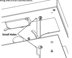
Step 5: Remove the outer sheathing of the Power Cable (E) and twist the outer conductor into a wire. This should be connected to the Black (–) driver lead with a wire nut. Strip the sheathing off the inner conductor. This should be connected to the Red (+) driver lead with a wire nut. Wrap each connection individually with electrical tape to ensure no portion of the conductor is exposed.
