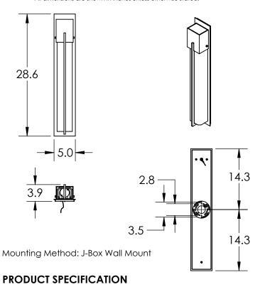
Construction: Aluminum Body With Formed Glass
