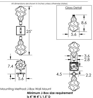
Construction: Aluminum Body, Blown Glass
