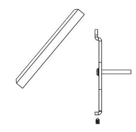
Step 4: Use #8-32 set screw (C) to fasten light in place.
